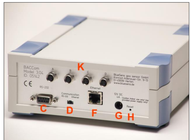
Abb. 32: Anschlüsse am BACCom12
